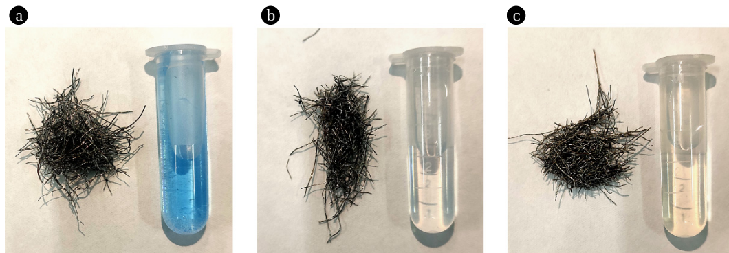
Fig. S2. The macroscopic images of brass-coated steel wires and corrosion solution after (a) AH corrosion, (b) after ammonia corrosion alone (20%), and (c) after hydrogen peroxide corrosion alone (10%). The corrosion time is 5 min
