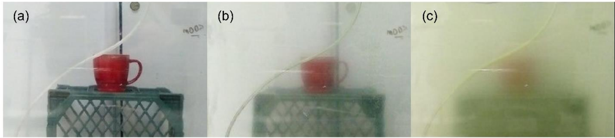
1 2 Fig. 3. Variation of color and transparency of the green window. (a) Before microalgae culture; 3 (b) After 12 h of microalgae culture; (c) After 180 h of microalgae culture.
